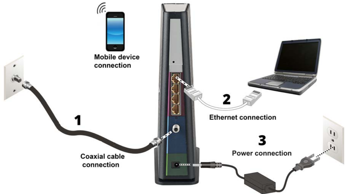
Figure 4: SBG8300 connection diagram
